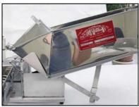
9. The "pig" is used for boiling and cooling the syrup for the product (see MAKING MAPLE CANDY on page 6 and MAKING MAPLE CREAM on page 8). When the syrup has reached the temperature for the product, the "pig" is placed on the "pig" platform. The "pig" platform has the same approximate shape as the "pig" so align the spout end of the "pig" toward the trough and slide the "pig" against the raised front edges of the platform
