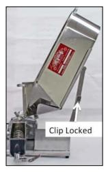
10. Slowly raise the platform and "pig" until the hinge locks. NOTE: There will be weight and possibly hot surfaces dependent on the product and quantity being processed.
