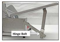
8. Hold the "pig" platform and push the hinge at the bolt carefully away from the machine base. Lower the "pig" platform slowly until the hinge won't move any further.
