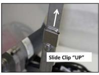
7. Support the "pig" platform and slide the locking clip on the "pig" holder hinge up.
