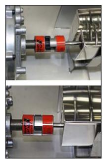
5. Line up the coupler at the end of the worm with the open spots in the spider and slide the trough down into the holders on the base. Slide the trough until the worm spiral end is just touching the spigot end of the trough. There should be no back and forth motion of the coupler joint.
