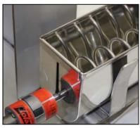
6. Put the slide gate inside the end of the trough where the worm shaft slot is cut. Slide the gate down until it is seated on the edge of the trough.
