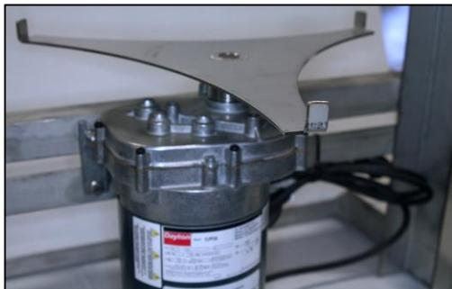
2. Place the pan on the cream machine. Align the pan with the tabs of the base. The cream machine turns clockwise
