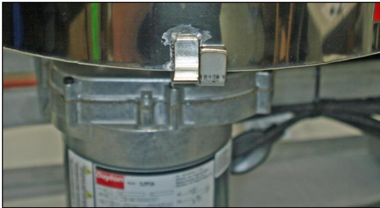
6. Place the pan with the cooled syrup onto the cream machine base. Line the pan up with the holder. The motor turns clockwise so align the tabs on the pan to the left side of the tabs on the holder. This will prevent slipping and wear when the motor starts.
