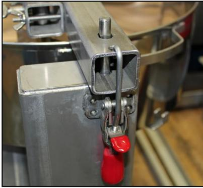
3. The top of the paddle bar has two holes in each end. Insert the paddles into the paddle holders on the paddle bar. The top of the paddle rod should be on the same side as the top of the paddle bar
