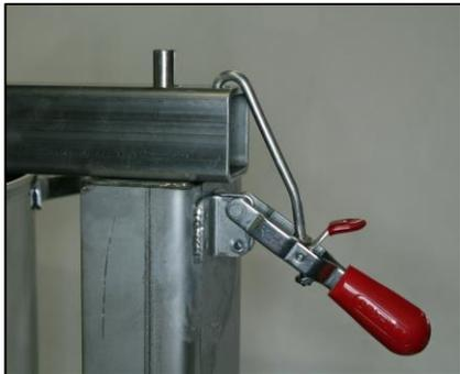
4. Position the paddles about 1/2" from the bottom of the paddle bar then tighten the thumbscrew to hold the paddles. Place the paddle bar on the base pins. Lock the paddle bar in place using the snap locks inserted into the outer holes on the top of the paddle bar.
