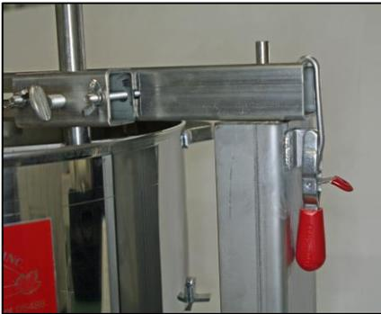
5. Install the outer paddle (the one with the projection of the bottom). The outer paddle holder slot (in the paddle bar) is the one that opens furthest to the outside for the pan
